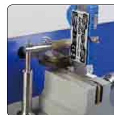
lapping measuring surfaces of caliper lower jaws
